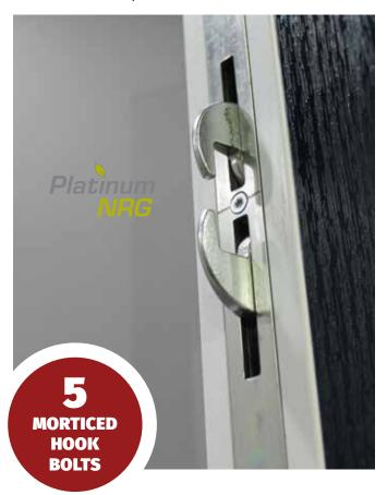
Each standard door consists of 5 morticed Hook Bolts. There are two at the top of the door, one in the centre and a second pair at the bottom. Each of these pairs work together to hook towards one another and ensure that not only can they deter entry by force, they are able to stop any attempt to lever the door apart - in any direction!
